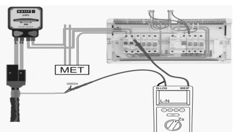
Note:-Combined green/black test lead, part no 328A954 is required for 2 wire measurements.
