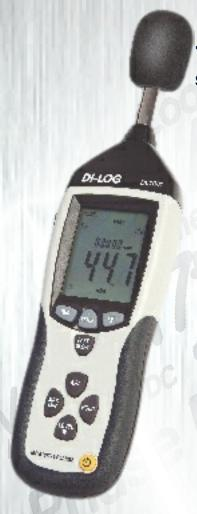
The DL7031 Class 2 digital sound level meter is a professional meter for measuring noise levels in conformance with IEC 61672-1 class 2 with a highly accurate range of +/- 1.4dB
