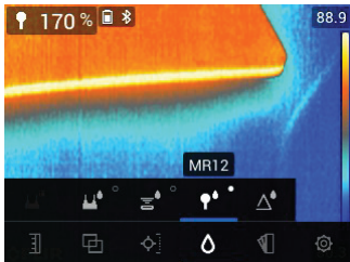
Figure 5.20 Selecting the MR12 (optional moisture probe) mode
